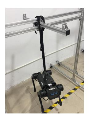
In addition to the bracket, 1 nylon rope will be used to suspend the robot.
